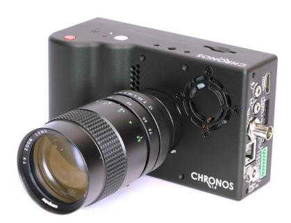
Chronos 1.4 is a 1.4 gigapixel-per-second handheld high-speed camera. Completely self-contained, you can take high-speed imaging with you anywhere. It records 1280x1024 video at 1057fps, and can record at up to 38 500fps at lower resolution. Video is saved in compressed h.264 or uncompressed RAW format to removable media. You can shoot for hours, saving hundreds of shots on a single card.
