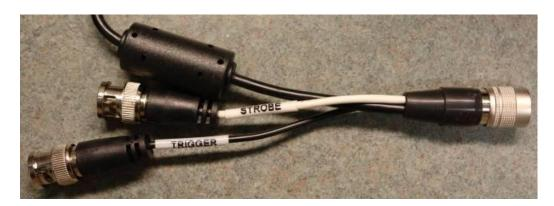
Trigger & Strobe pigtail with Male BNC connectors
