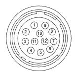
Figure 1.9 – HD-SDI Camera Power Connector Pin-Outs (Rear view).
